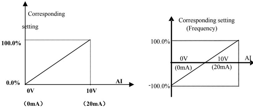
Fig 6-14 correspondence of analog input to setting
