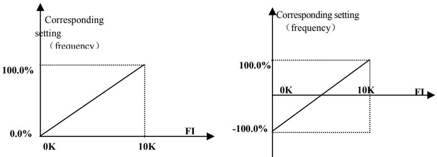
Fig 6-15 correspondence of pulse input and setting
