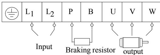
Power terminals sketch of inverter with 3-phase 230V 1.5kW and below 1.5kW.
