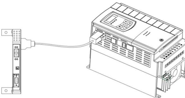
Fig 9-11 connection between communication card and inverter
