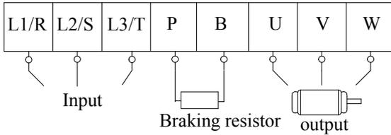
Power terminals sketch of inverter with 1-phase 230V 2.2kW, 3-phase 230V 2.2kW~5.5 kW, and 3-phase 400V 0.75kW~15kW.
