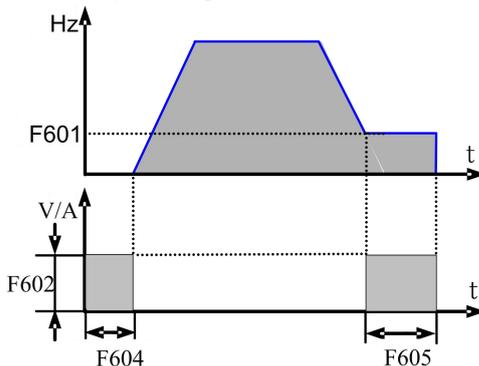
Figure 6-19 DC braking
