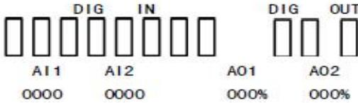
The first line indicates digital input, digital output; First eight boxes in the second line indicate the state of DI terminals, terminals from left to right are DI1~DI8, solid-line box is the state showed as above when terminal is invalid; Black box is displayed when terminal is valid. E.g. If all 8 terminals are valid, **■■■■■■■■** will be displayed.
