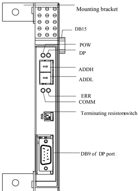
Fig 2-2 Communication card appearance and structure component
