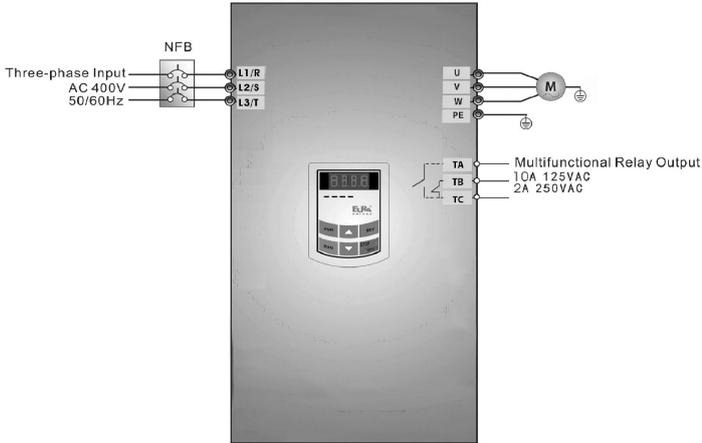
Figure 5-7 Wiring Diagram 1
