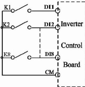
**2. Wiring for active source electrode**
