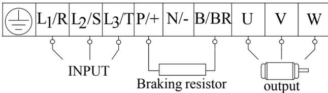
Power terminals sketch of inverter with 3-phase 230V 15~75kW and 3-phase 400V 55kW~185kW hanging type inverter and 110kW~160kW cabinet inverter.
