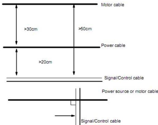
Generally, the control cables should be shielded cables and the shielding metal net must be connected to the metal enclosure of the drive by cable clamps.
