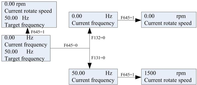
Fig 5-4 Operating flow chart of status parameter display
