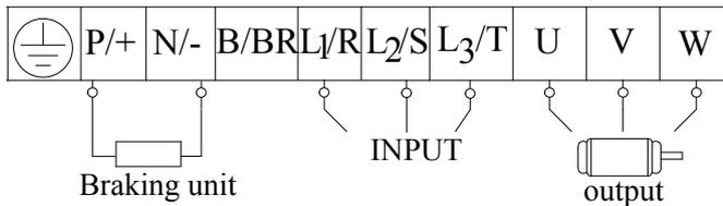
Power terminals sketch of inverter with 3-phase 200kw~400kw hanging type inverter and 185kw~800kw cabinet inverter.
