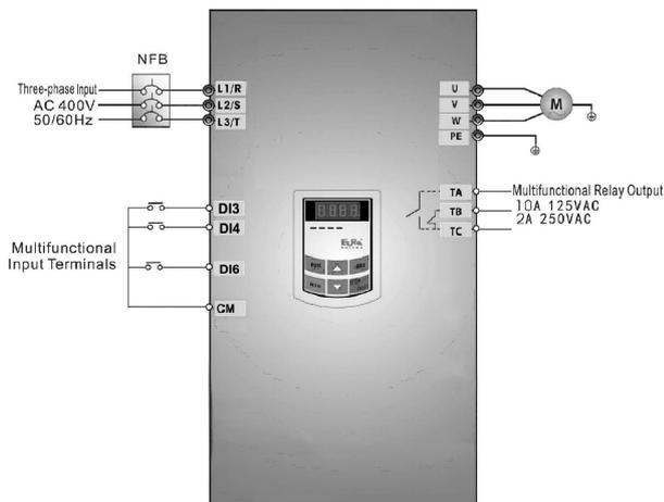
Figure 5-8 Wiring Diagram 2
