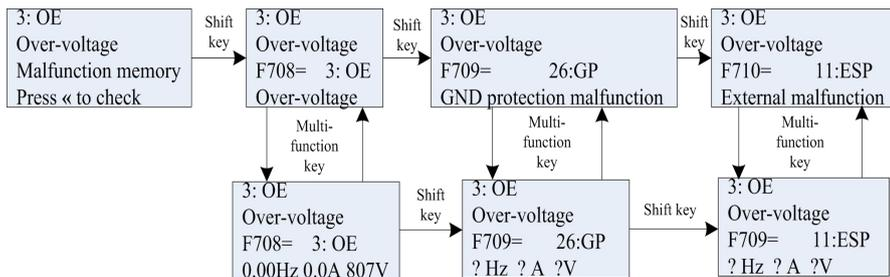
Fig 5-6 Operating flow chart of displayed malfunction interface
