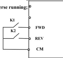
2. Two-line mode 2: when this mode is used, FWD is enable terminal, the direction is controlled by REV terminal.
