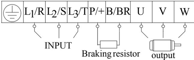
Power terminals sketch of inverter with 3-phase 230V 7.5~11kW and three-phase 400V 18.5kW~45kW.
