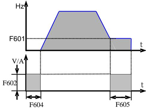
**Figure 5-18 DC braking**
